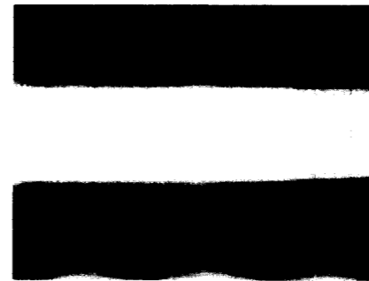
TP1 (REC LEVEL) MODE:REC 10mVX10/div 2msec/div (MCV-C P.C.B)
